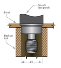
For installations in most aluminums or low carbon steels that are ¼ hard or softer
